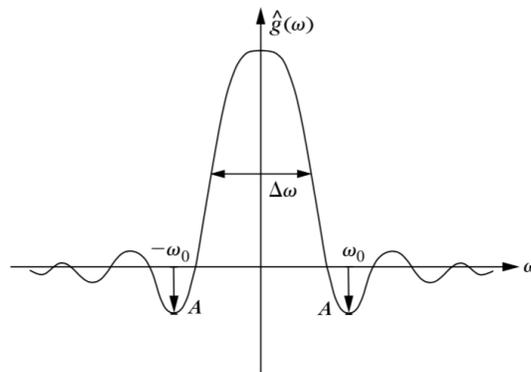
Figure 10: The energy spread of  $\widehat{g}(\omega)$  is measured by its bandwidth and the maximum amplitude  $A$  of the first side lobes, located at  $\pm\omega_0$ .
